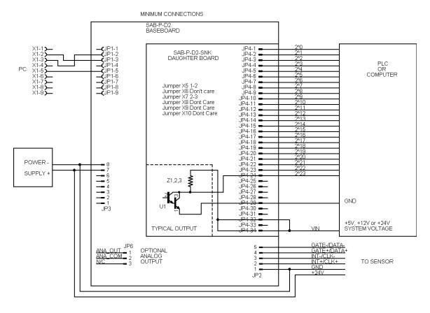
Sensor may be isolated by using a separate power supply.
